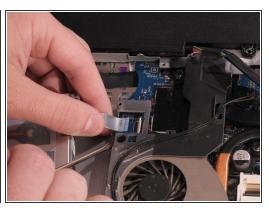
Carefully disconnect the connecting cable by lifting the white clamp with a Flathead screwdriver and pulling on the blue tab away from connector.
