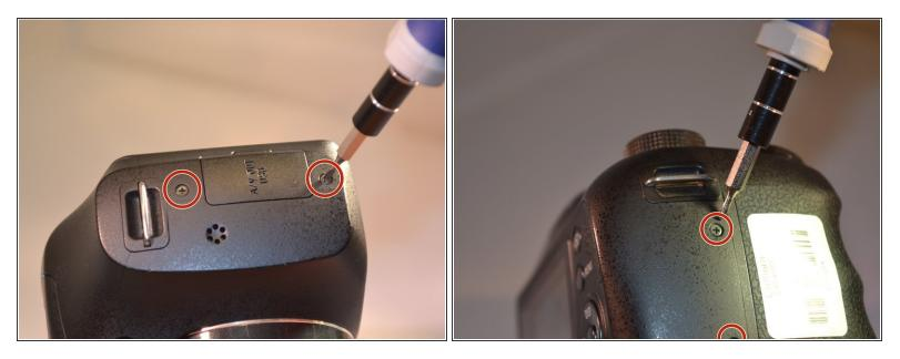
• Using a screwdriver, remove four 6mm screws located on the back panel.
