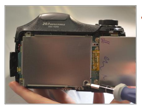
Using a screwdriver, remove the single 4mm screw at the bottom of the holding plate.
