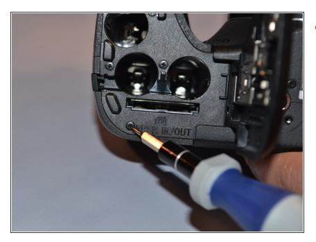
Open the SD Door, unscrew and remove the single 6mm screw closest to "PUSH IN/OUT" under the SD card slot.
