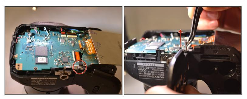
Using tweezers remove the pin that attaches the door to the body.
