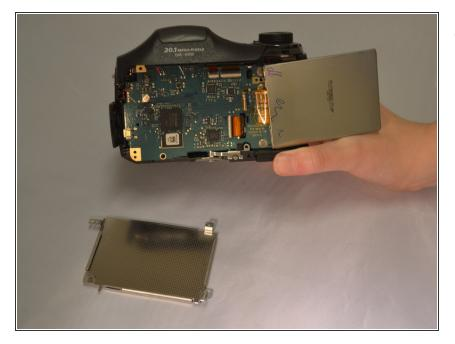
• Lift the holding plate away from the motherboard and set aside (the pin attaching the door to the body is now accessible).
