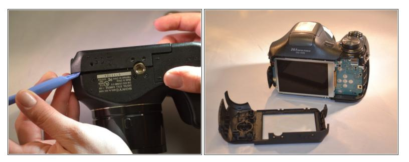
Using the blue plastic opening tools, remove the back panel (the LCD and motherboard are exposed).
