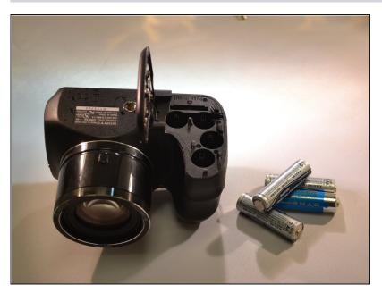
Take the four AA batteries out of the battery compartment.
