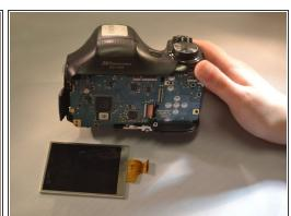
• Using tweezers, remove the LCD with the ribbon cable and set aside.
