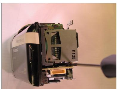
Remove the black 4 mm screw located on the back of the camcorder under the SD card slot.
