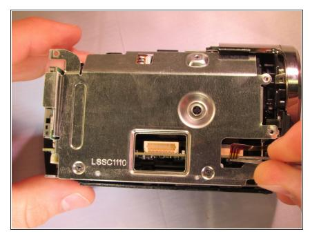
There is a small copper ribbon on the right side of the device. Pull gently with the tweezers upward from the right side to get the copper ribbon free.
