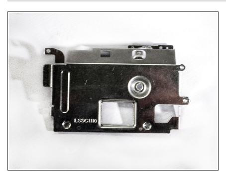
Pull the metal casing straight off (The metal casing will be detached from the rest of the device).
