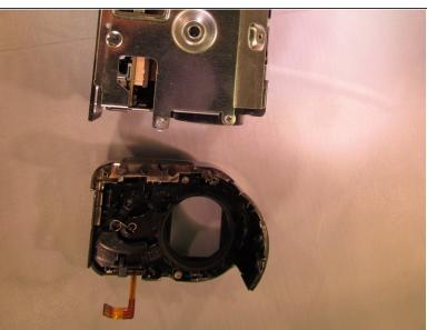
Pry upwards on the front cover from the top of the device and with your other hand pull straight out on the front of the device (The front cover will be detached and free).
