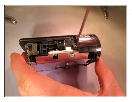
Unscrew the silver 4 mm screw from on top of the camcorder.
