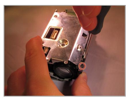
Remove the 6 mm screw on the top of the metal casing which was under the front cover.
