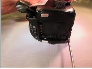
Remove the black 4 mm screw from the back of the camcorder underneath where the battery would have been.
