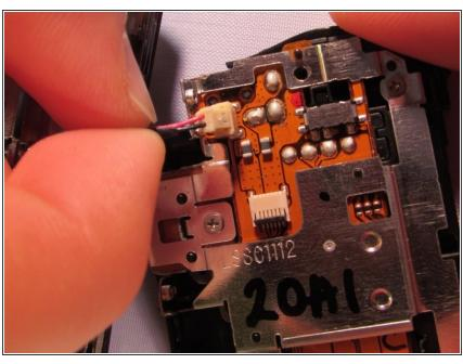
Gently pull on the red and black wires directly outwards so that these wires become detached.
