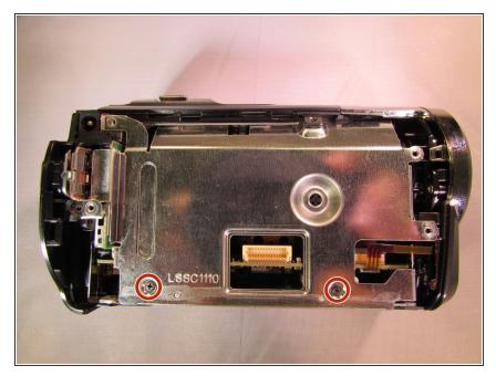
Unscrew the two black 4 mm screws from metal casing around the motherboard.
