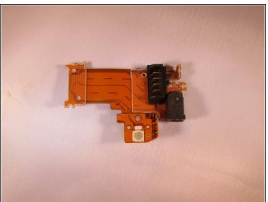
Pull up gently on the larger orange piece. Then, gently pull out the piece to release it from the plastic back panel. The charging port is now ready to be replaced.
