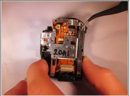
Push in on the tab and lift the metal bracket. Remove the metal bracket from the back panel.
