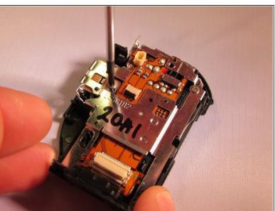
Unscrew the two silver screws on the back panel as seen in the image.
