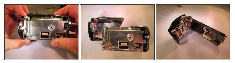
• Pull the plastic cover on the back out and up slightly until the back feels like it's free, then pull back on the plastic (The top cover piece and back will be detached).
