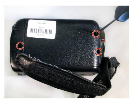
• Remove the three 6-mm screws on the hand-strap side of the camera.
