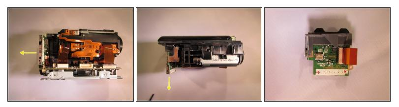
Pull the SD card slot slightly to the side and detach the SD card slot (the SD card slot is ready to be replaced).
