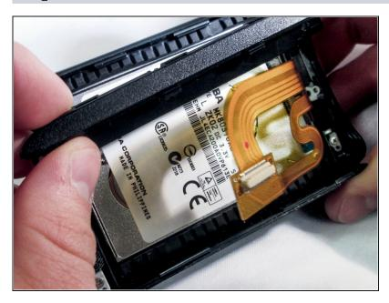
Gently pull the black plastic hard drive case away from the body of the camera. This will expose the hard drive (HDD).
