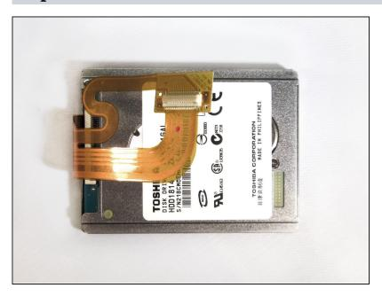
The HDD has been removed and ready to be replaced.
