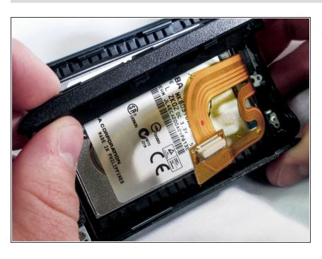
Gently pull the black plastic hard drive case away from the body of the camera. This will expose the hard drive (HDD).
