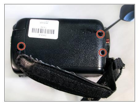
Remove the three 6-mm screws on the hand-strap side of the camera.
