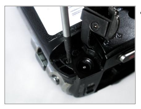
Pull out the charging port (DC input terminal) cover and remove the 4mm screw located next to the input terminal.
