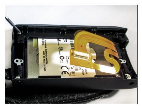
Remove the two 4 mm silver screws located on the HDD casing.
