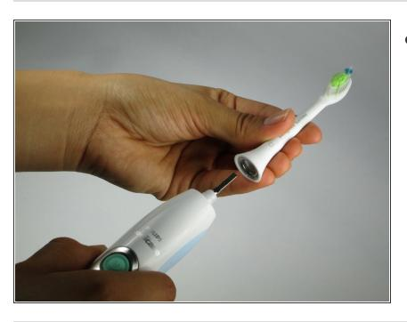
Once the hands are placed in the correct positions, carefully separate the two by pulling them apart.
