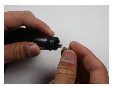
Turn the charger compartment over and carefully dump the fuse into your hand.
