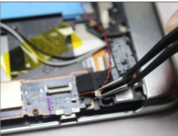
Remove the red and black cable using the tweezers by gently pulling the connector to the right.
