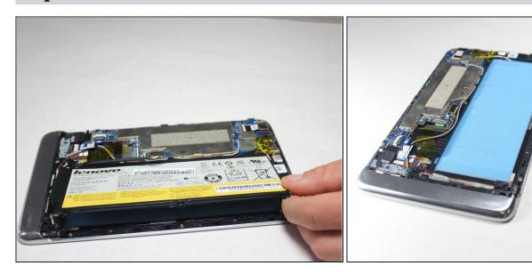
• Remove the battery by prying up with your fingers or a plastic opening tool.
