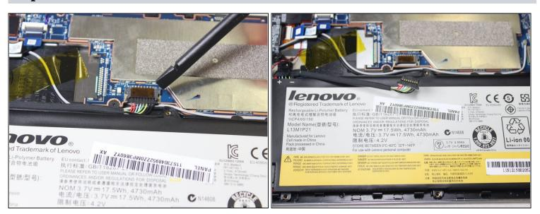
Using a plastic spudger, slowly push each side of the battery connector (back and forward a couple of times) out of its socket on the motherboard.
