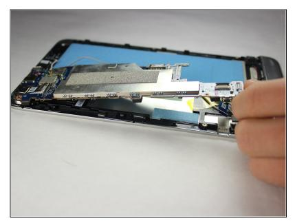
• Lift the motherboard out of the tablet's case.
