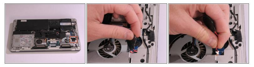
• Unplug CMOS battery by gently pulling upwards on it's cable.
