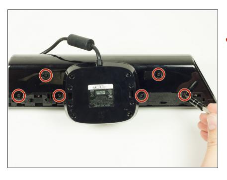
Unscrew the six 12mm T10 Torx screws.
