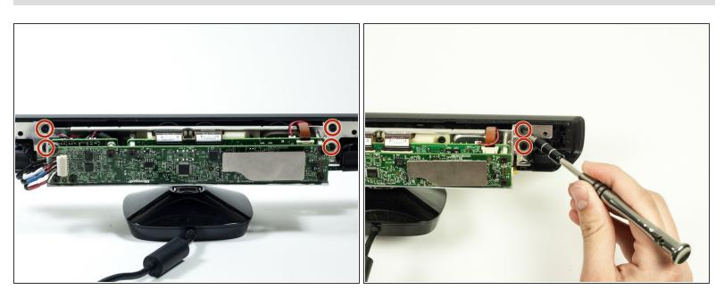
Remove the four 7mm T10 Torx screws (two on each side of the metal body).
