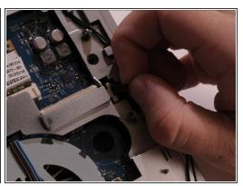
Remove the second connector by gently pulling upward.
