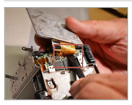
Using spudger, lift the tab on the connector and remove the orange ribbon from motherboard (LCD screen is separated from camera).
