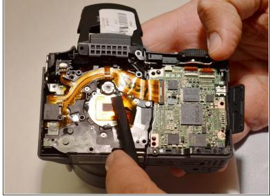
• Using the spudger, lift the tab on the ZIF connector and remove both orange ribbons connected to the green motherboard (Motherboard is lifted from camera).
