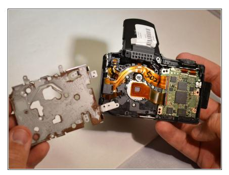
Using the spudger, remove the metal housing (Metal housing is removed from camera).
