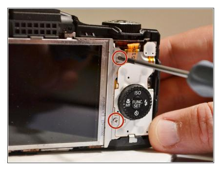
Using the Phillips 00 screwdriver, remove the two 3mm screws closest to the right of the LCD screen.
