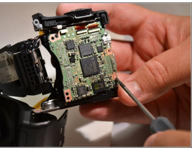
Using the Phillips 00 screwdriver, remove the 4mm screw from motherboard.
