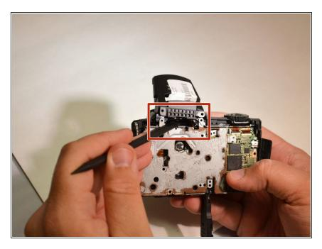
Using the spudger, lift the flash unit away from the metal housing (Flash is lifted to allow more room for metal housing).
