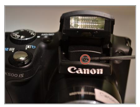
Using the Phillips 00 screwdriver, remove the 4mm mounting screw from underneath the flash.
