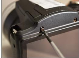
Using the Phillips 00 screwdriver, remove the two 4mm top screws above the LCD screen.
