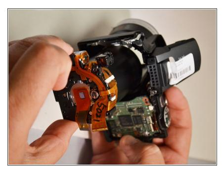
Remove the lens from the lens shaft (Lens is removed from camera).
