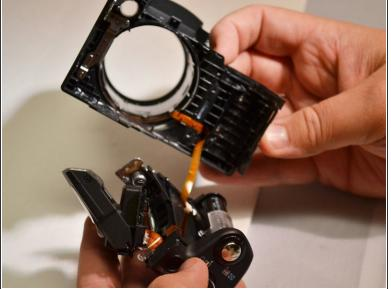
Using the plastic pry tool, remove the motherboard and the flash unit from camera frame (Motherboard and flash unit are separated from camera).
