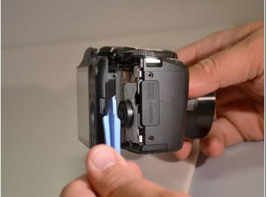
Using the plastic pry tool, remove the back cover from camera.
