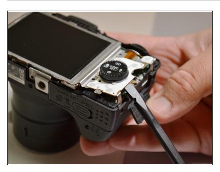
Using the spudger, lift the control dial to the right of the LCD screen.
