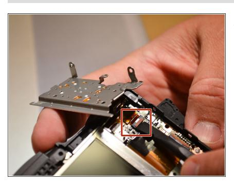
Using the spudger, lift the connection tab and remove the control dial's orange ribbon from motherboard.
