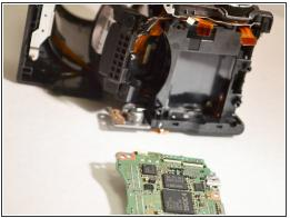
• Using the plastic opening tool, lift the tab on the connector and remove the two remaining orange ribbons from green motherboard (Motherboard is removed).
