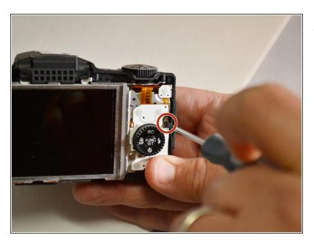
Using the Phiillips 00 screwdriver, remove the 4mm screw to the right of the control dial.
