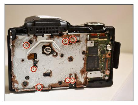
Using the Phillips 00 screwdriver remove the seven 6mm screws from the housing plate of the LCD screen.
