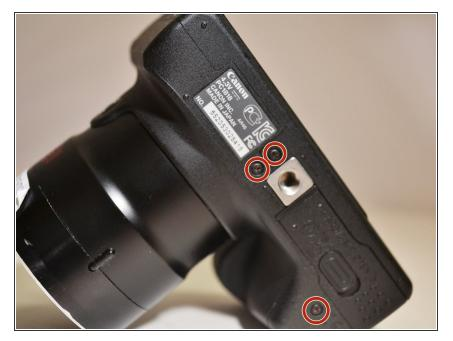
Using the Phillips 00 screwdriver, remove the three 4mm screws from the underside of the camera.
