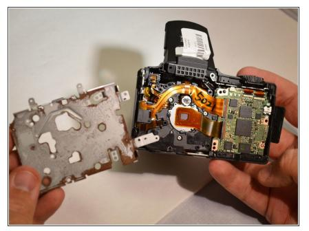
• Using the spudger, remove the metal housing (Metal housing is removed from camera).
