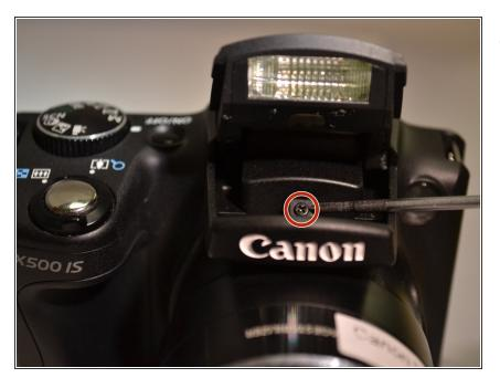
Using the Phillips 00 screwdriver, remove the 4mm mounting screw from underneath the flash.
