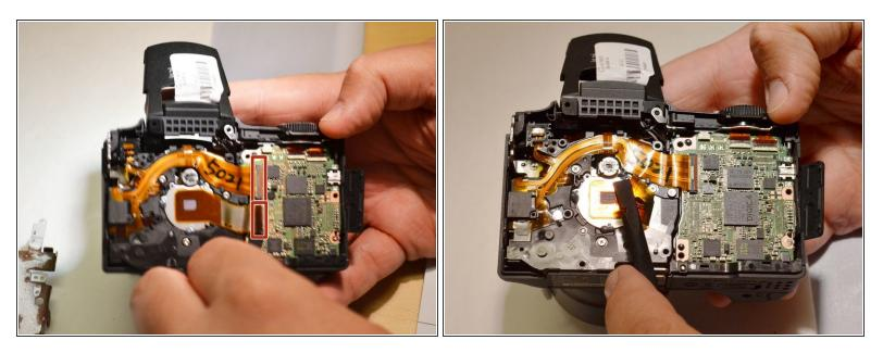
Using the spudger, lift the tab on the ZIF connector and remove both orange ribbons connected to the green motherboard (Motherboard is lifted from camera).
