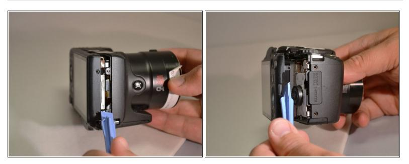
• Using the plastic pry tool, remove the back cover from camera.
