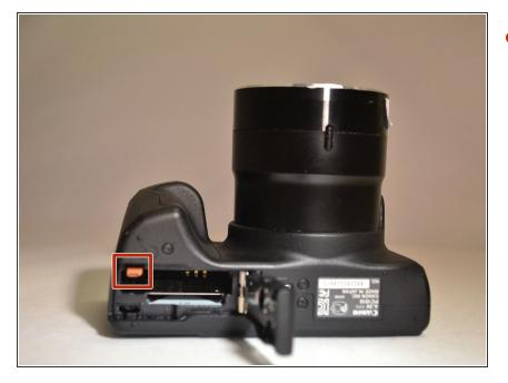
Push the small orange tab forward to release the battery (Battery is ready for removal).
