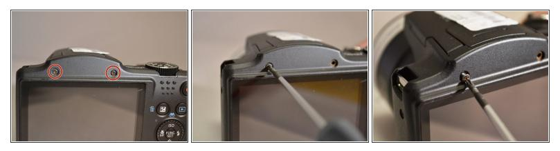
• Using the Phillips 00 screwdriver, remove the two 4mm top screws above the LCD screen.
