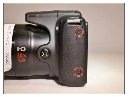
Using the Phillips 00 screwdriver, remove the two 4mm side screws to the left of the LCD screen.
