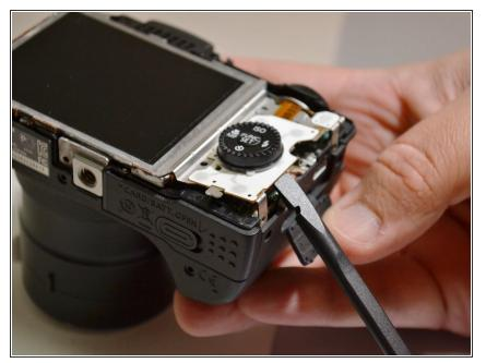
• Using the spudger, lift the control dial to the right of the LCD screen.
