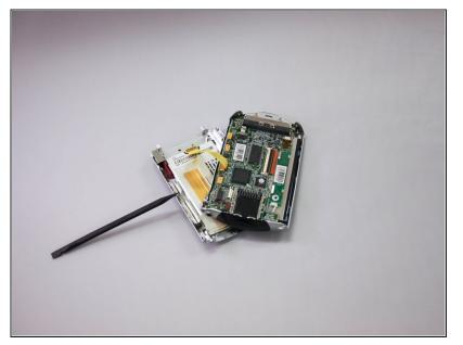
• Carefully remove the back cover using a plastic opening tool against the grooves along the sides of the iPAQ.
