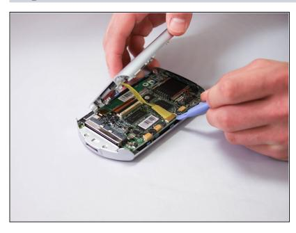
At this point, a yellow ribbon will be connecting both the front and back panels of the device. Carefully use the plastic opening tool to detach the ribbon from the connector pins.
