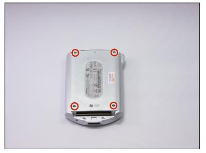
• Remove the four screws found on the back cover of the device.
