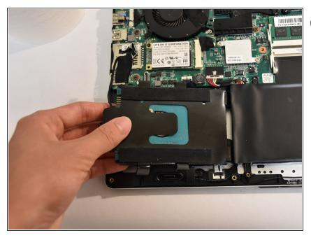
*i* Carefully lift the hard drive for removal.
