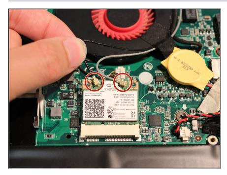
Remove the black and grey wires that are connected to the wireless card by pulling away from the card.
