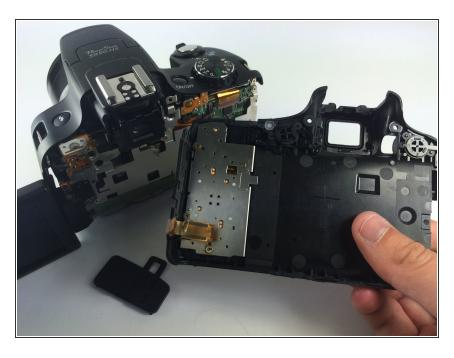
Now you can completely separate the back encasement from the rest of the camera.
