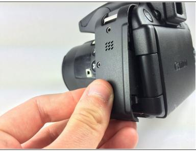
Use the plastic opening tool to carefully start lifting up the camera's left-side panel. Then use your fingers to pry off the rest.
