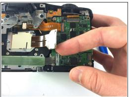
Remove the two wire ribbons on the bottom left corner of the I/O board by unclipping them with your fingers.
