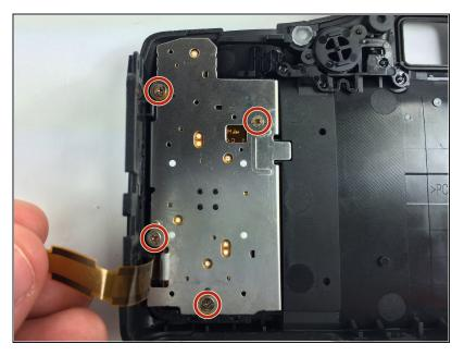
• Remove the four Phillips #000 screws, length 3 mm, attaching the metal panel to the inside of the back encasement.
