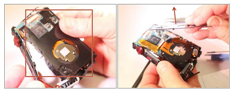
After the LCD screen has been removed there is a black metal plate that can be pulled off revealing the motherboard and the lens.
