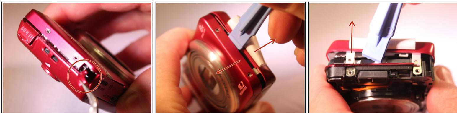
**i** Take note of the small free moving flap near the battery port seen in the first of the three photos. Be sure to store the free moving flap in a safe place.
