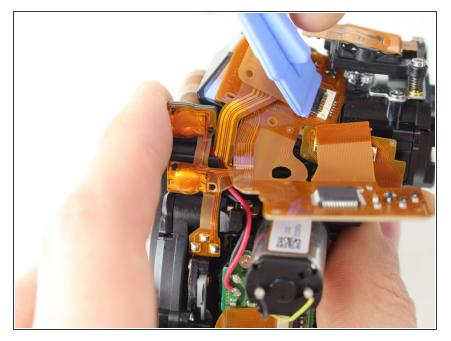
Disconnect ribbon cable at top right of camera.
