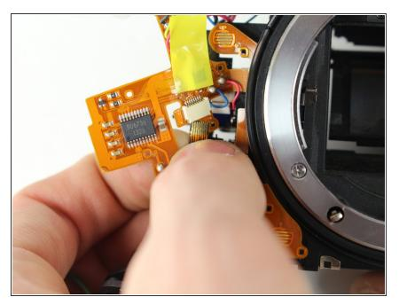
• Pull out ribbon cable from circuit asembly near front left of device.
