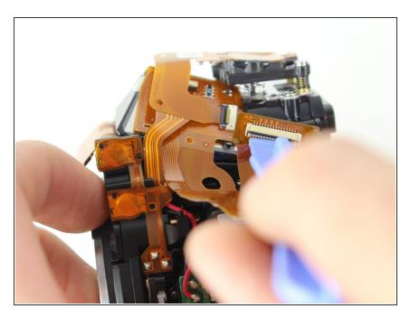
• Disconnect ribbon cable at the top right of camera.
