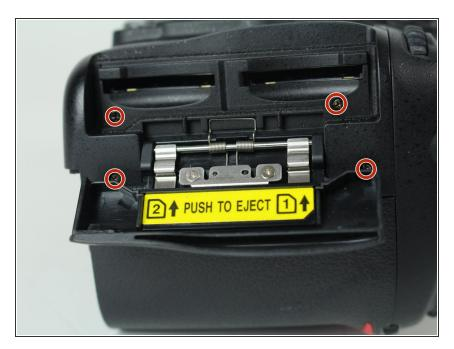
• Remove four 6 mm J000 screws that secure the SD card cover.
