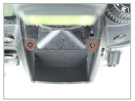
• Remove two 5 mm J000 screws from under the flash.
