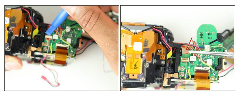
• Remove the left front ribbon cable from top right of circuit board.
