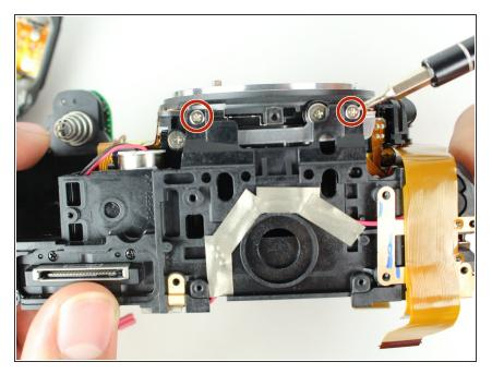
Remove two 6.5 mm J000 screws from beneath the lens mount.
