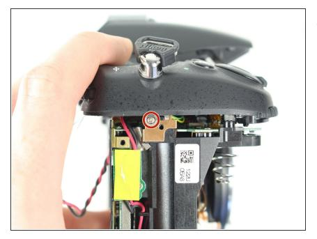
Remove one 4 mm J000 screw securing the top case (under left strap hook).
