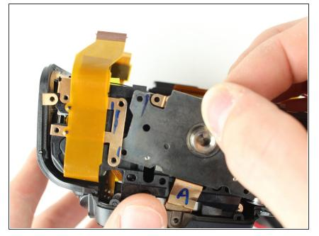
• Carefully lift the tripod plate from the backside of the camera and slide out the grounding clip from under the lens mount.
