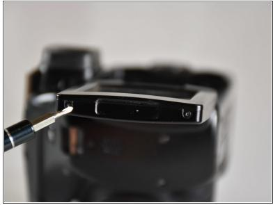
Unscrew the two 3 mm screws shown on the left side of the LCD screen panel using a Phillips screwdriver.
