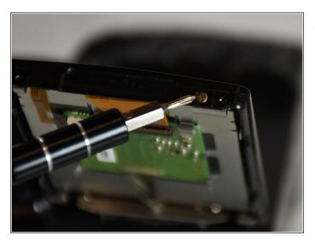
Unscrew the 2mm screw on the outer edge of the panel
