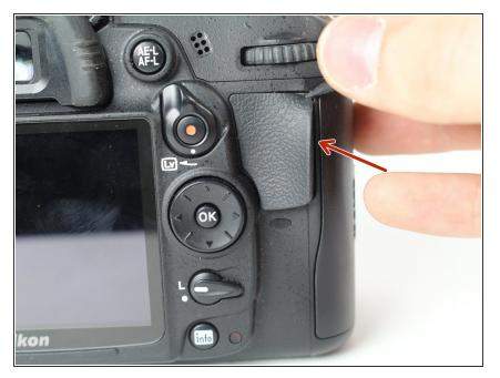
• Peel the rear rubber piece off with tweezers.
