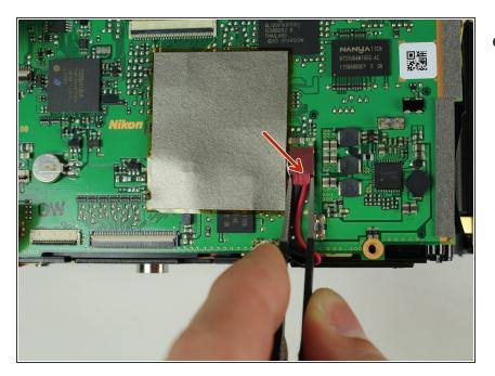
• Carefully disconnect the red connector with tweezers.
