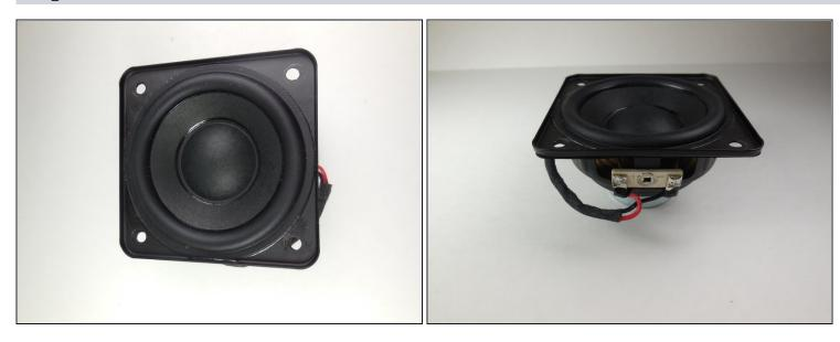
• The subwoofer has now been removed from the device and can be replaced.
