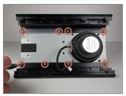
Remove eight 8 mm Phillips #2 screws holding the subwoofer tray to the housing.
