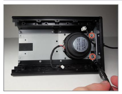
Remove two 8 mm Phillips #2 screws holding the side panel in place.
