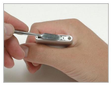
• Use a metal spudger to carefully pry the headphone jack out of the casing. DO NOT remove the headphone jack from the iPod entirely, as it is connected via a fragile ribbon connector to the click wheel.
