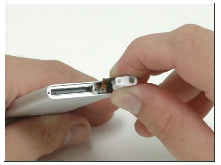
Slide the headphone jack out until the white plastic housing is no longer held in place by the metal casing.
