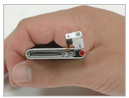
Remove the newly-revealed Phillips #00 screw from beneath the headphone jack.
