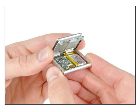
Remove the rear panel from the Shuffle.
