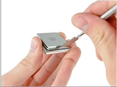
• Use a combination of iPod opening tools and metal spudgers to pry the rear panel away from the Shuffle by the seam nearest the ON/OFF switch.
