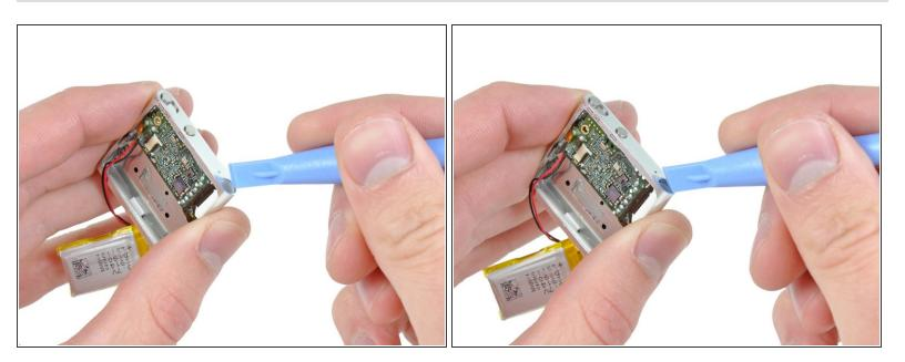
Use the edge of an iPod opening tool to push the headphone jack down toward the center of the Shuffle.
