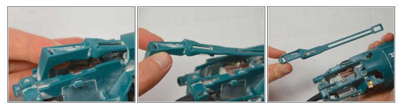
• Pull the switch lever up and out of the body of the angle grinder.
