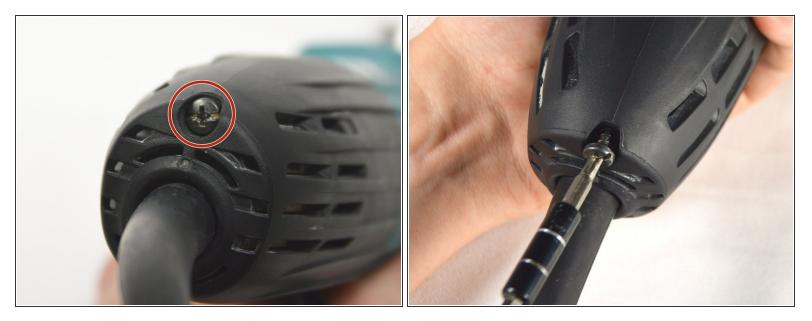
• Unscrew the 20 mm tapping screw using a Philips #02 screwdriver.
