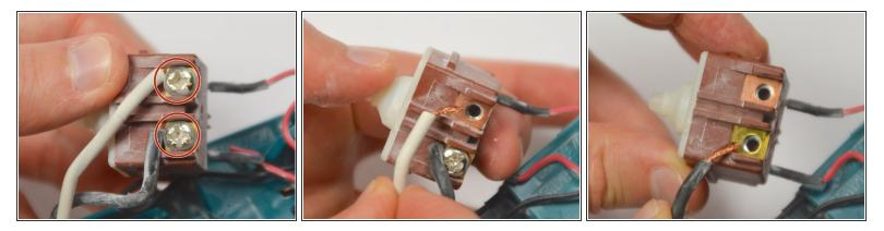
Remove the two 10 mm screws holding the power cord leads in place using a Phillips #02 screwdriver.
