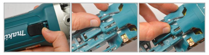
• Place your finger in the gap in front of the switch. Now, at the base of the device, push the switch lever into the 'on' position.
