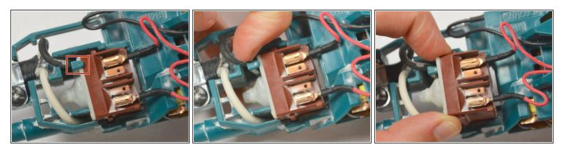
• Pull back the plastic clip and pull the internal switch up and out of the cavity.
