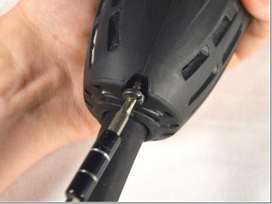
• Unscrew the 20 mm tapping screw using a Philips #02 screwdriver.
