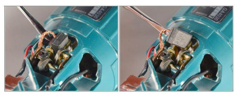
Using a metal spudger, remove both carbon brushes (one on each side) by their copper cabling.
