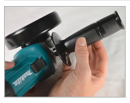
Unscrew the handle unit until it is removed completely.
