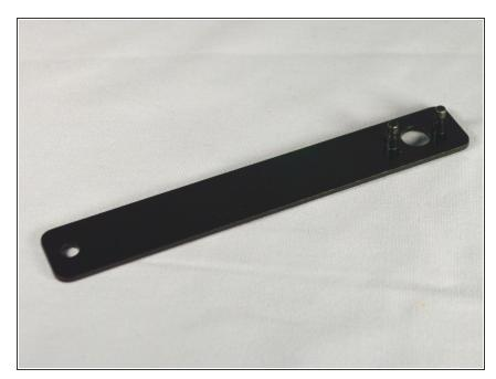
Check for the provided lock nut wrench. This is used for loosening the piece that keeps the disk and cover attached.
