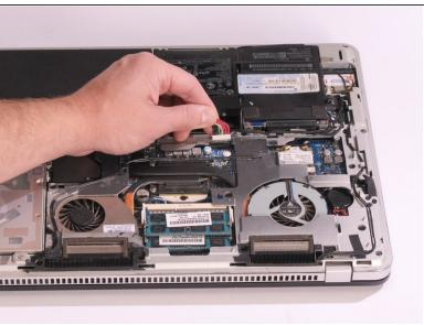
• Disconnect the multi-colored battery cable from the main assembly by gently pulling upward on it.
