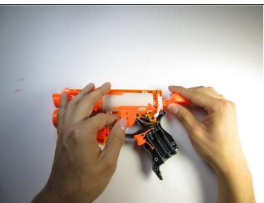
Remove the firing trigger by grabbing the trigger with your fingers and pulling it up and out.
