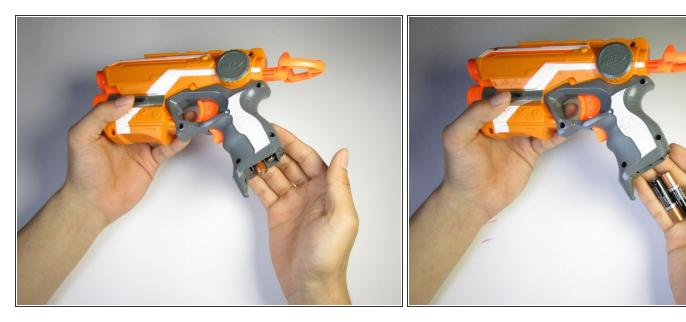
Slide out the two AAA batteries using your fingers.
