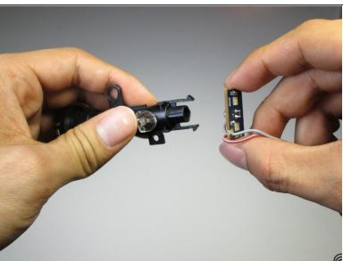
Pinch the clips holding the circuit board to the laser assembly and remove the circuit board.
