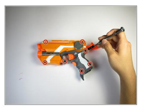
Remove the seven 10-mm black Phillips screws from the blaster casing with a #1 Phillips Screwdriver.
