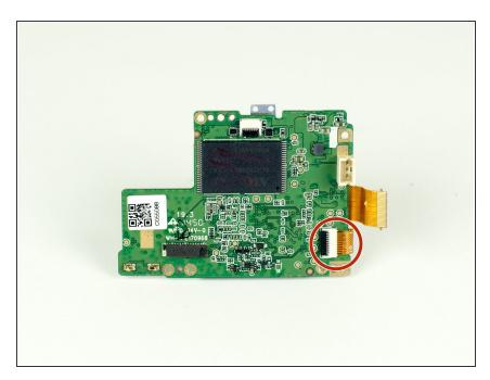
Remove the ribbon cable from the motherboard by simply pulling the cable from the socket.
