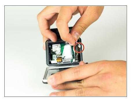
Disconnect the battery from the motherboard by unplugging the red, white, and black wires from the white adapter.
