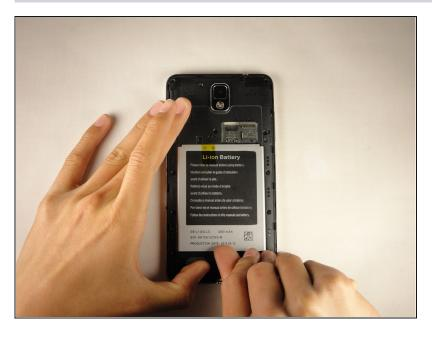
Remove the battery by placing your thumb in the slot, pushing the battery up and pulling it out.
