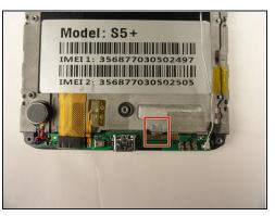
Remove the silver tape that holds the lower motherboard to the front panel of the phone.
