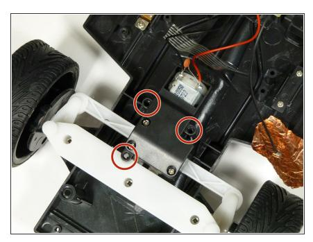
Remove the three 1.6mm Phillips #000 screws from the black motor casing.
