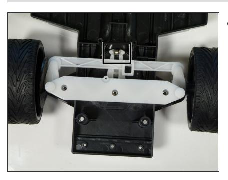
Carefully remove the steering column spring.
