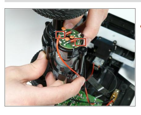
Use a soldering gun to remove the attached wires To reassemble your device, follow these instructions in reverse order.
