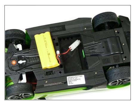
Unplug the battery by pushing on the clip.
