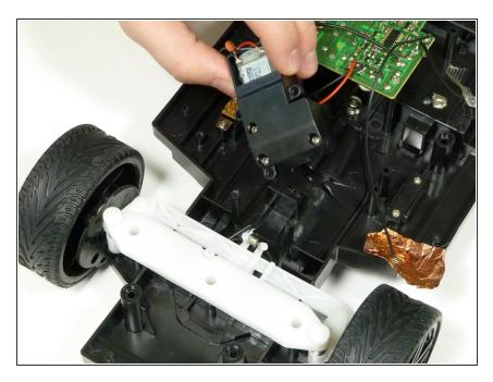
Remove the front motor and its casing from the chassis of the car.
