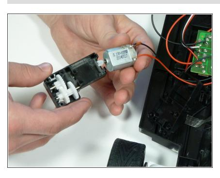
Pull out the front motor, making sure to keep the gears intact To reassemble your device, follow these instructions in reverse order.
