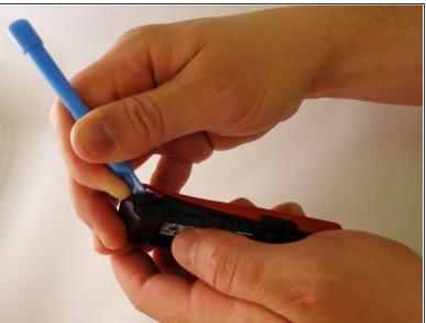
Insert the prying tool between the seam of the faceplate and the body.
