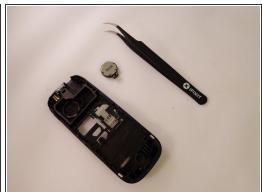
Insert tweezers into the small crevices of the backside of the speaker, and lift upwards.
