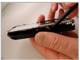
Using the spudger, pry back three tabs located on the left edge and three tabs located on the right edge of the body.
