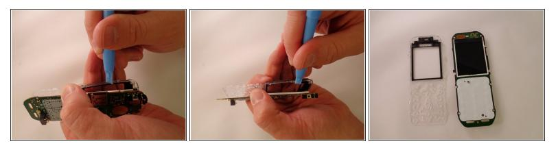
• Insert the prying tool between the tabs and the motherboard. Loosen and separate slowly.
