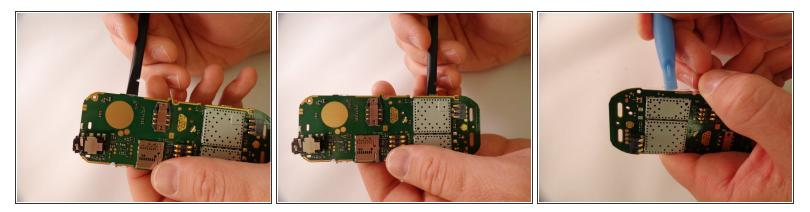
• Locate the four clear tabs that connect the screen to the motherboard.
