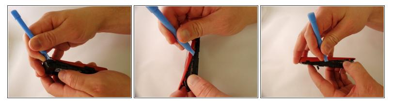
Starting from the bottom of the phone, begin prying around the base of the phone alternating form left to right.
