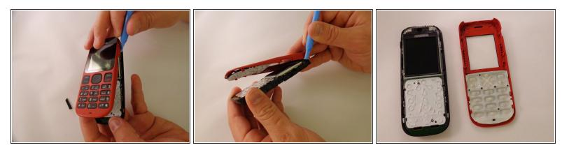
As the base loosens, slowly increase the separation between the plates and the body of the phone.
