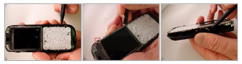
Using the spudger, pry back three tabs located on the left edge and three tabs located on the right edge of the body.
