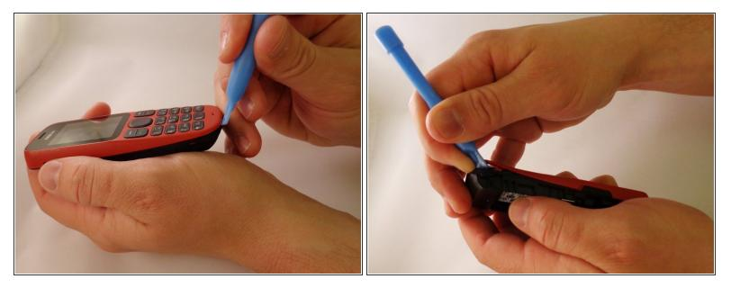
• Insert the prying tool between the seam of the faceplate and the body.
