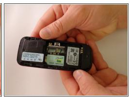
Using the prying tool, pull back the latch of the SIM Card holder.
