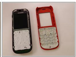
As the base loosens, slowly increase the separation between the plates and the body of the phone.
