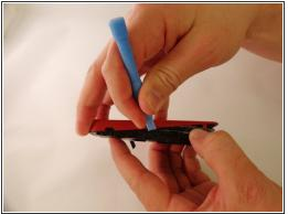
Starting from the bottom of the phone, begin prying around the base of the phone alternating form left to right.
