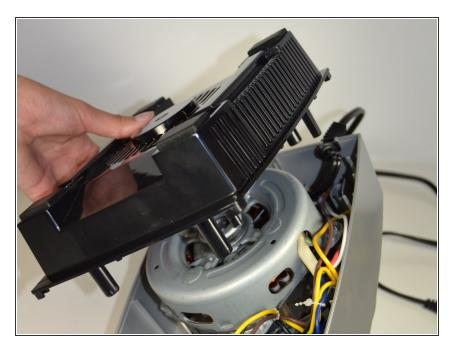
Remove the bottom casing of the food processor and set aside.
