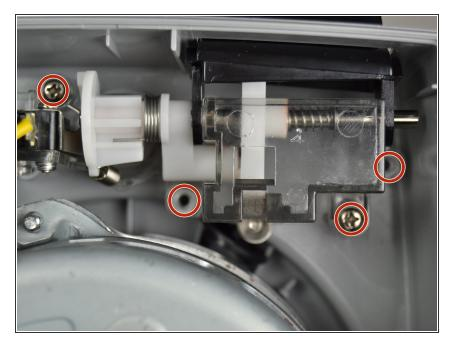
Remove the four screws (circled in red) holding the switch down.
