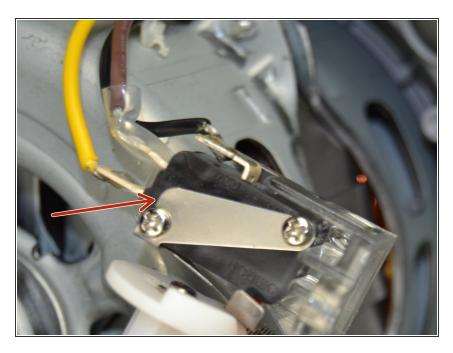
Remove the component (shown by the arrow in the picture to the left) attached to wires from the switch.
