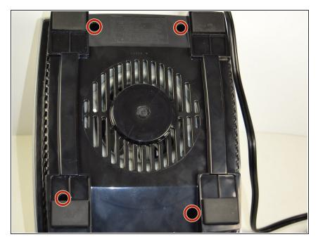
Remove the four screws (circled in red) out of the bottom of the processor using a Philips #2 Screwdriver.
