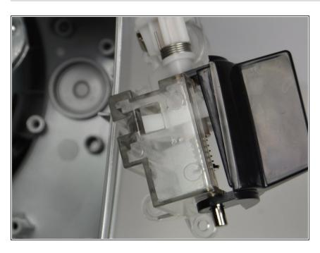
Carefully remove and replace the switch, now that the wires are detached.
