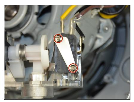
Remove the two screws from the switch (circled in red) attached by wires.
