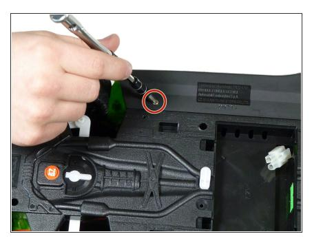
Unscrew the two 2.5mm Phillips #00 screws from each side
