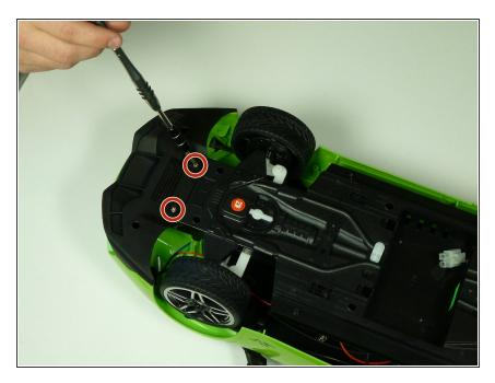
Unscrew the two 2.5mm Phillips #00 screws from the front skirt of the car.
