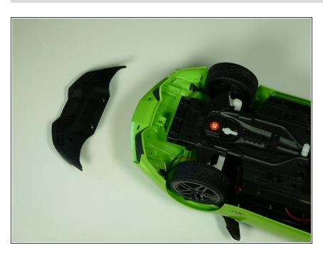
Lift the front part of the underbody and pull it out from the main underbody.
